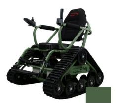
The Track Chair has a seat width of 22 inches and no maximum weight restrictions. Features include: Comfort Tek back, seat base, and armrest, 4 point harness, 9" seatbelt extension, armrest pockets, attendant control, flip up footrest to help with transfers, head rest, lateral leg supports, lateral side reports, oxygen tank holder, and transfer handle and backpack hook.
